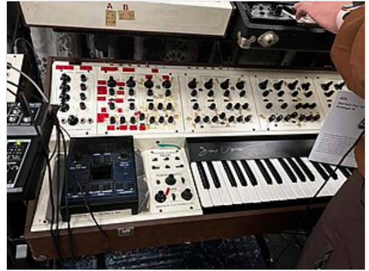
The first prototype of the Oberheim 4-voice synthesizer , as used by Wonder. The front panel still shows the braille labeling.
